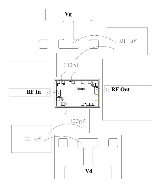
All three Vd pads (pad # 9, 10, 11 from mechanical drawing) do not need to be connected
