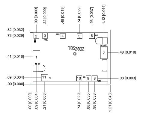
Units: millimeters [inches] Thickness: 0.10 [0.004] (reference only) Chip edge to bond pad dimensions are shown to center of bond pads. Chip size tolerance: ±0.05 [0.002] RF ground through backside
